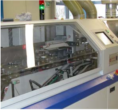
Inclining infeed channel and lifting table ensure smoothing transition of the book blocks into the clamps.
